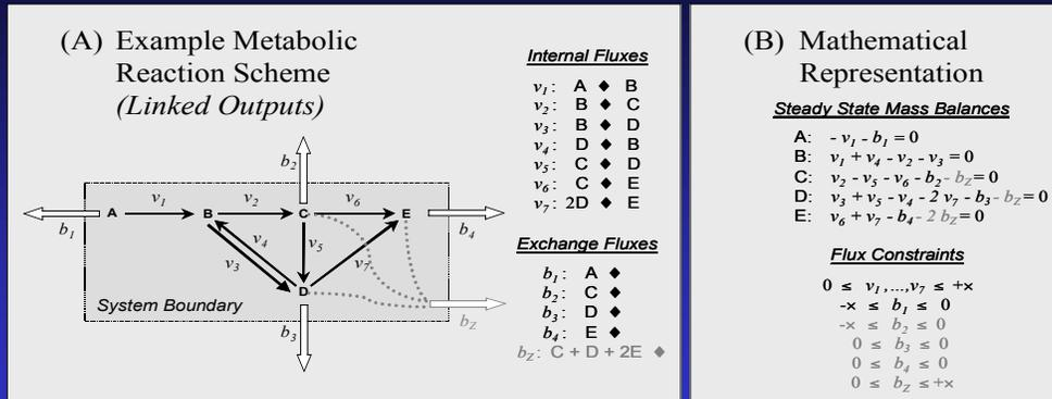
Metabolic reaction scheme with the addition of an aggregate demand flux taking one mole of metabolite C and D, and 2 moles of metabolite E. The corresponding changes to the mass balances and inequality constraints on the fluxes are indicated in gray type, representing the effects of linked outputs.
